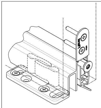
Planet SL assembly DIN R, with floor guide, release on lock side
