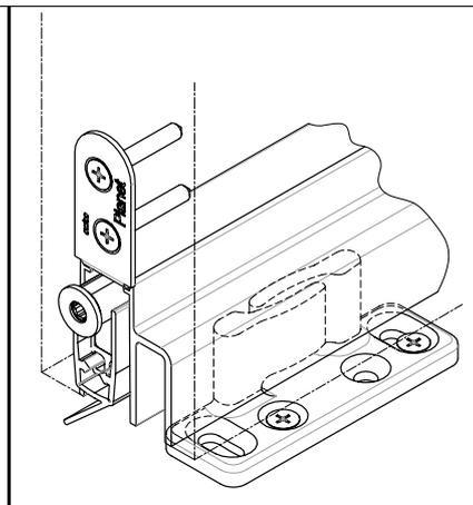
Planet SL assembly DIN L, with floor guide, release on lock side
