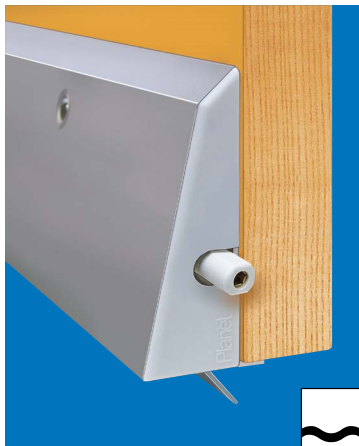
Planet Socle with Planet RF 13×30 mm, for heavy wavy floors, with covering plate and release knob
